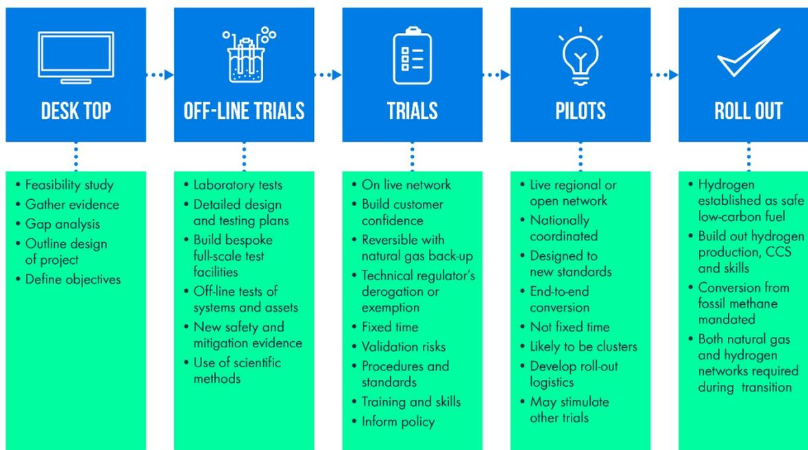
**Figure 20 Evidence pathway for decarbonisation of networks using hydrogen**
