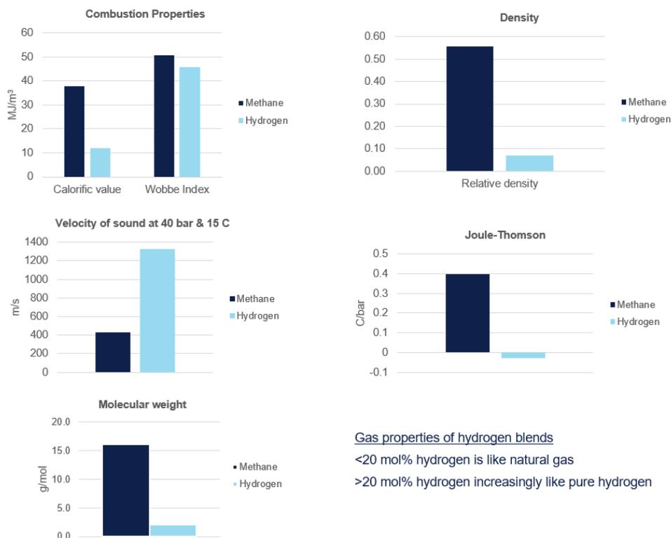
**Figure 21 Summary of the differences in the properties of typical natural gas and 100% hydrogen**
