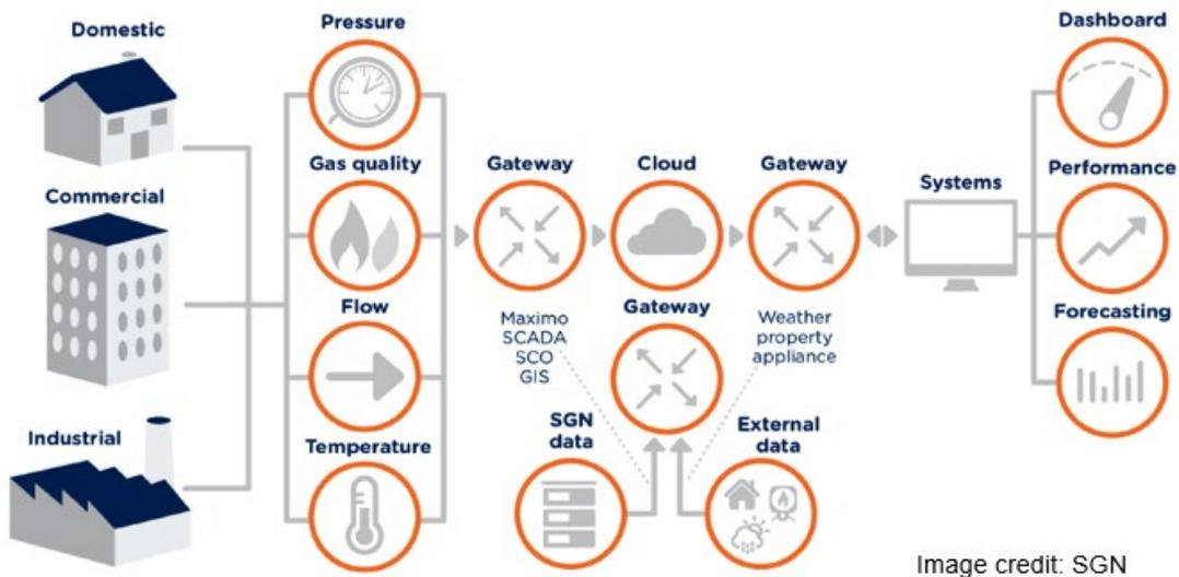
Figure 24 Data flow in the Real-Time Networks project.
